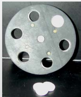
Figure 1. Hydroxyapatite disks used in the rotating disk reactor system.
